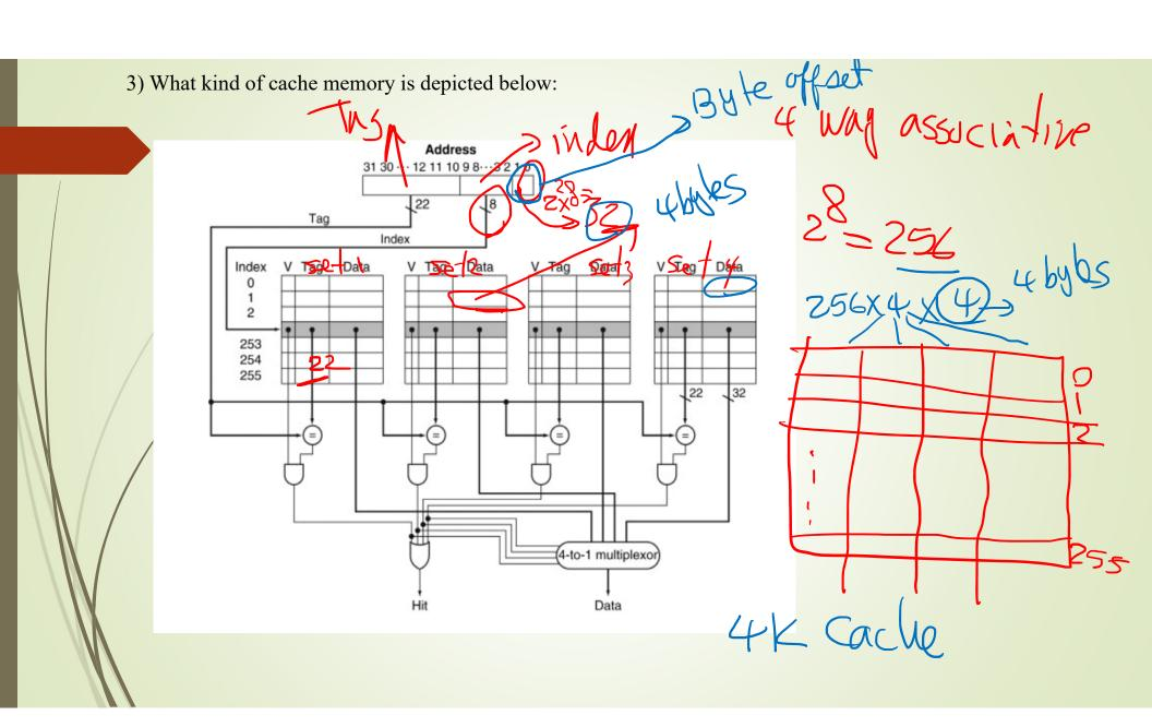
The \_\_\_\_\_ of every cache block within the appropriate set of a setassociative cache is checked for a match against the memory block address.
